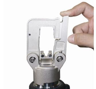
4. Slide the dies into the open head. Make sure the dies are matching and seated correctly.
