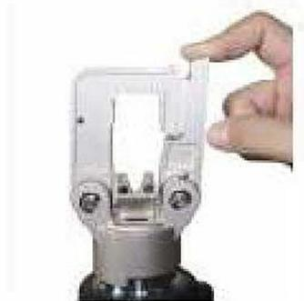
4. Slide the dies into the open head. Make sure the dies are matching and seated correctly.
