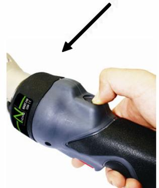
3. Pull back the latch to open the head. The head will spring open.
