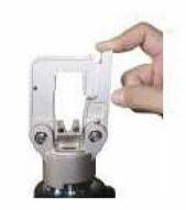
4. Slide the dies into the open head. Make sure the dies are matching and seated correctly.
