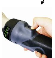
3. Pull back the latch to open the head, the head Will spring open.
